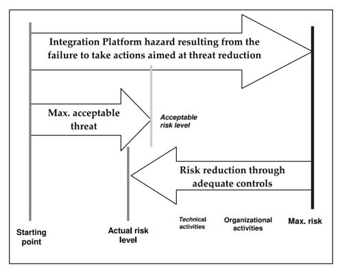
**Figure 2.** Illustration of the functional security principle Source: Own elaboration.
