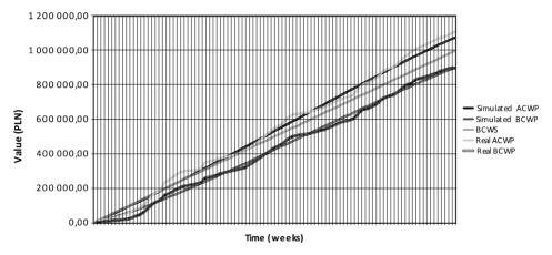
**Figure 2.** Comparison of the results generated by the simulation to the real project data Source: Own elaboration.
