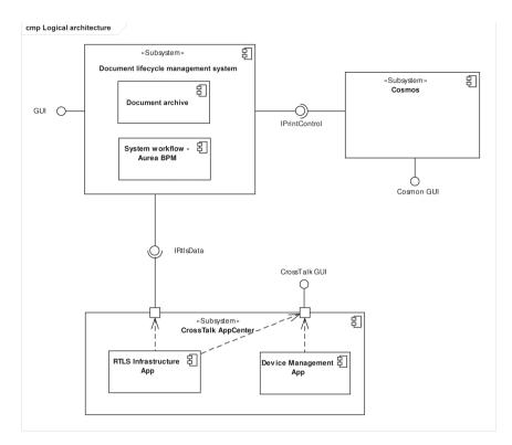
**Figure 26.2.** Logical architecture of the classified document lifecycle management system Source: Own elaboration.
